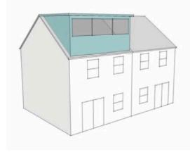
Box dormer is excessively scaled relative to the roof and has poor window alignment with those below.
